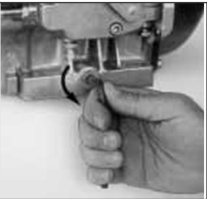
Remove drain plug and drain oil into an approved container. Reinstall drain plug.
